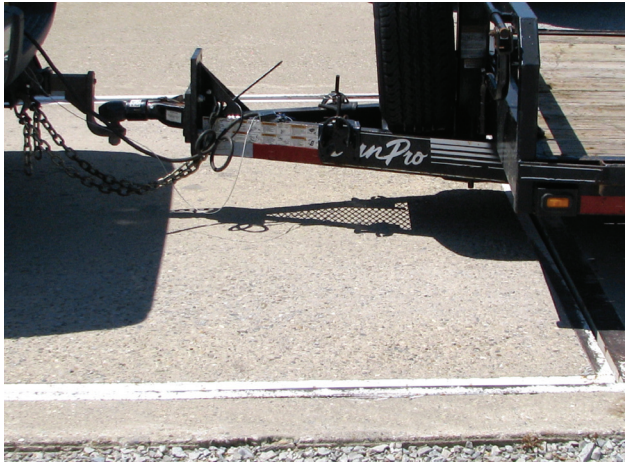
Weighing a trailer in the way shown here will produce a figure that includes tongue weight of trailer.
