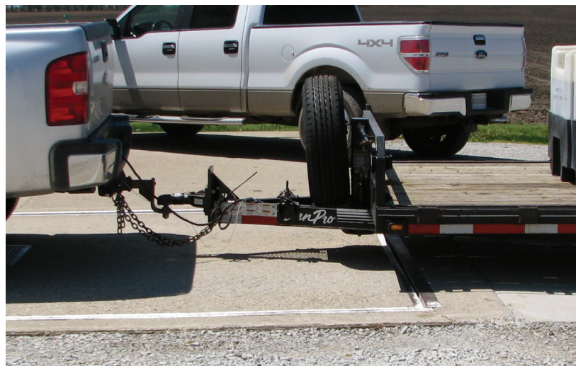
Weighing a trailer in the way shown here will produce a figure that includes tongue weight of trailer.
